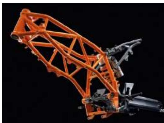
*Figura 2. 6. Chasis multitubular [44]*
