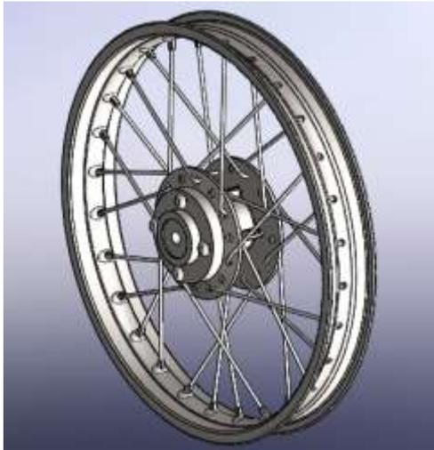
*Figura 2. 40, Modelo CAD Llanta delantera*
