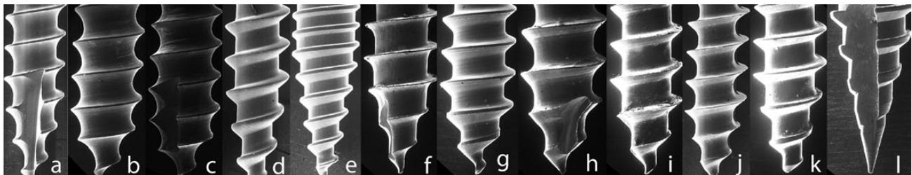
**Figure 1.** Scanning electronic microscope images of the used miniscrew types a: Thomas, b: Biomaterial Red, c: Biomaterial Pink, d: Novaxa, e: 3M, f: Dewimed, g: Osstem, h: Jeilmed20, i: Jeilmed16, l: Forestadent, m: Aarhus, n: Storm.
