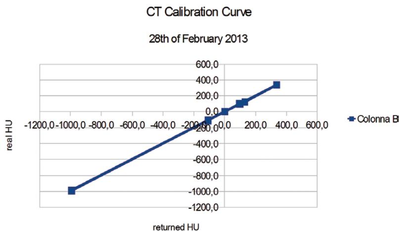
Figure 10. CT calibration curve (scanning objects of known density).
