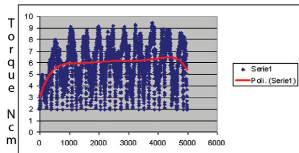
Figure 3. Insertion torque values (Ncm) according to time acquisitions (60 registrations per second).
