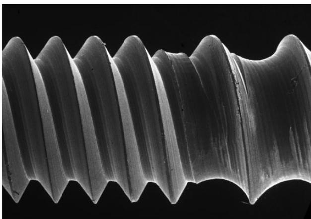
Figure 9. SEM image of double-threaded region in Biomaterial Red and Pink screws.
