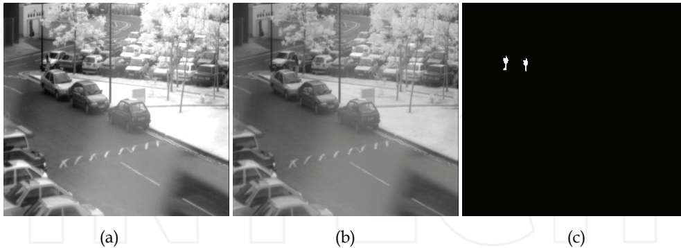
Fig. 16. Two consecutive scenes (a) and (b) of a captured sequence of frames from a car park scene. In (c) the object of interest is shown for the 2 scenes after detection algorithms have been applied.
