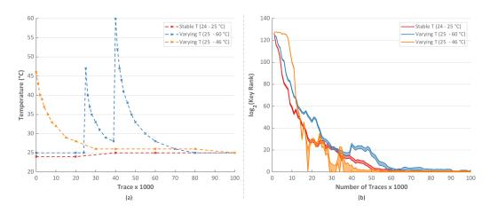
**Figure 11:** Results - Ambient Temperature. Shown in (a), Temperature Variation Pattern; and (b), Variation in KR over Number of Power Traces.
