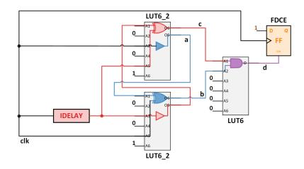
Figure 5: Implementation of Logic Gate Network on LUTs.
