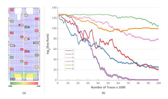
**Figure 8:** Results - Placement of PPWM. Shown in (a), Heat Map Based on Attack Efficacy; and (b), Variation in KR over Number of Power Traces.
