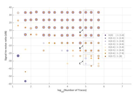
Figure 15: Impact of the Power Consumption Threshold.
