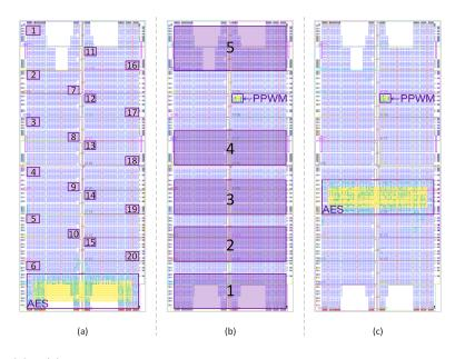
**Figure 7:** (a) - (c) PPWM and AES Module Placements on the Floorplan of SAKURA-G Main FPGA Used in Experiment Setup I.
