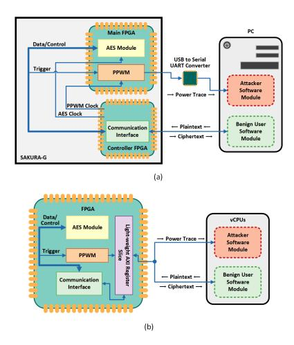
Figure 6: Diagram of (a), Experiment Setup I; and (b), Experiment Setup II.
