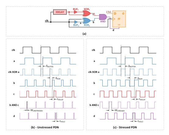
**Figure 3:** Working Principle of PPWM Sensor Showing (a), Labelled Block Diagram; (b), Waveforms for Unstressed PDN; and (c), Waveforms for Stressed PDN.
