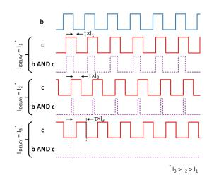
Figure 4: Calibrating t<sub>IDELAY</sub> with CONTROL\_FSM.
