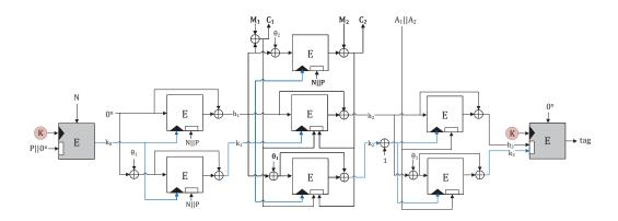
**Figure 7:** Triplex's full encryption details. The first 3 TBC calls on the left represents KDF producing the initial state  $(h_1, k_1)$ . The last TBC call on the right represents TGF producing the tag. Only the TBC calls colored in gray at the extremities are protected.
