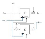
Figure 3: Hirose's compression function that is built on top of a tweakable block cipher E.
