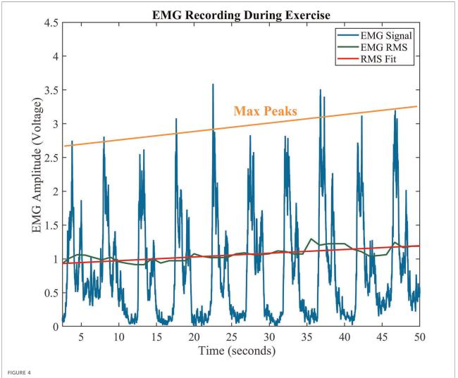
Amplitude vs. Time EMG Signal. Typical progression of EMG during exercise shows an increase in contraction peaks. The orange line shows a regression fitting of the peaks, while the solid green line shows the EMG RMS, and its best linear fit (red line).
