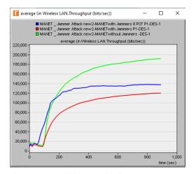
Fig. 10. Throughput (30 nodes, 8 PCF nodes, Transmission Power=0.001 W)
