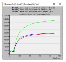
Fig. 12. Throughput (30 nodes, 8 PCF nodes, Transmission Power=0.01 W)
