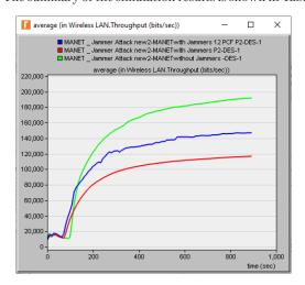
Fig. 16. Throughput (30 nodes, 12 PCF nodes, Transmission Power=0.01 W)
