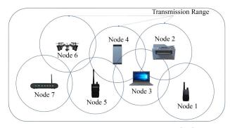
Fig. 1. Mobile ad hoc network topology [17]
