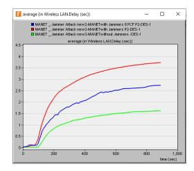
Fig. 13. Delay (30 nodes, 8 PCF nodes, Transmission Power=0.01 W)
