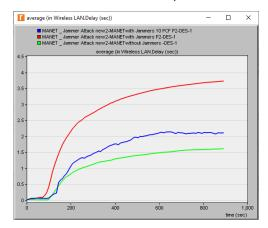
Fig. 15. Delay (30 nodes, 10 PCF nodes, Transmission Power=0.01 W)
