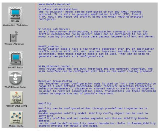
Fig. 5. Mobile ad hoc network types in Riverbed Modeler
