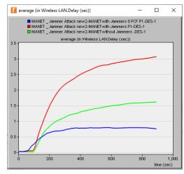
Fig. 11. Delay (30 nodes, 8 PCF nodes, Transmission Power=0.001 W)
