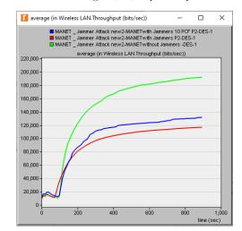
Fig. 14. Throughput (30 nodes, 10 PCF nodes, Transmission Power=0.01 W)
