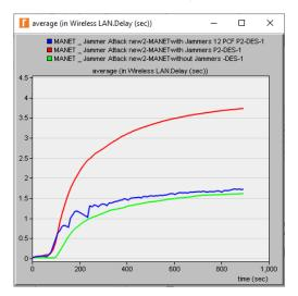
Fig. 17. Delay (30 nodes, 12 PCF nodes, Transmission Power=0.01 W)
