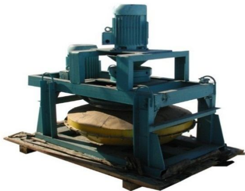
Fig.3. General view of the CMVU-800 mill
