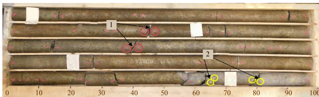
Fig. 1. Core of rich sulfide ore in contact with gabbro-dolerites
