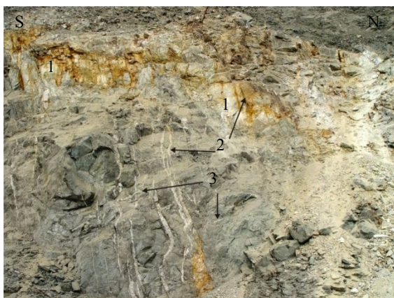
Fig.4. Types of quartz veins in the Svetlinsky quarry 1 – sub-meridional zone of secondary quartzite and adjacent quartz veins (in the image plane); 2 – sub-latitudinal quartz veins; 3 – sub-meridional small west-dipping veins
