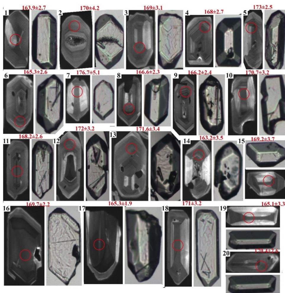
Fig.6. Montage of cathode luminescent (CL) and optical images of 20 studied zircon crystals from plagioryholites of the Monakh Cliff, Cape Fiolent. For each image, its number is indicated in black in the upper left corner. The position of the crater (circle, diameter 20 \mu\text{m} ) and the obtained age estimates (Ma) with a measurement error of 1\sigma are shown in red
