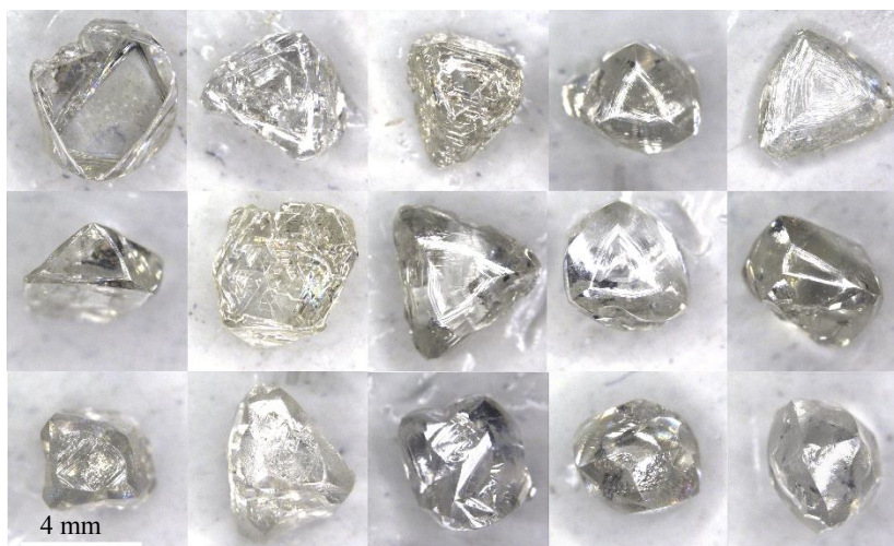
Fig.1. Typical in terms of morphology crystals of Arkhangelskaya and Karpinsky-I kimberlite pipes with different degrees of dissolution
