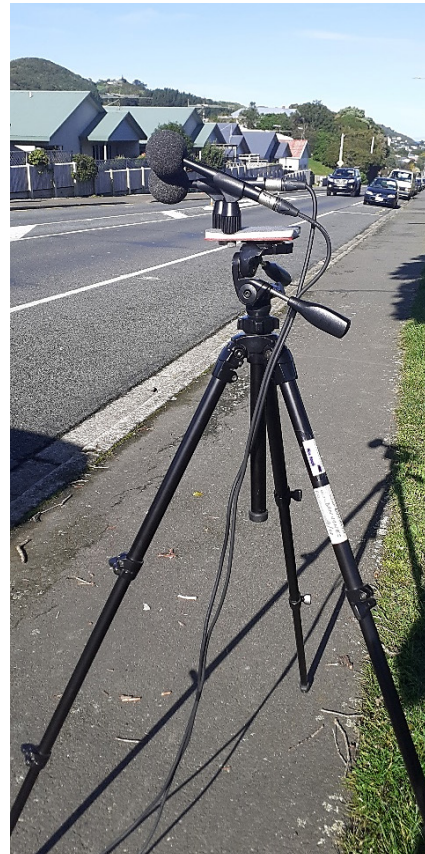
Figure 2. Microphones setup on a custom mounting plate on a tripod with windshields in place
