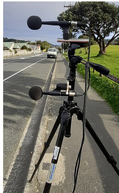
Figure 6. Microphone setup with the top one at 1.5 m and the lower at 1.2 m off the ground
