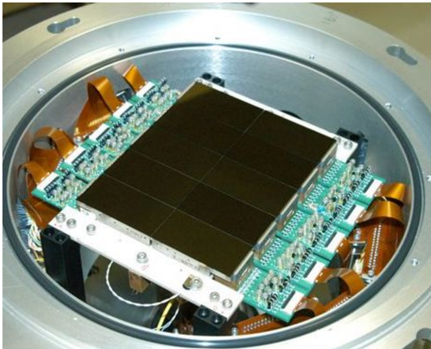
Figure 3.2: CCD arrangement for MOA-cam3
