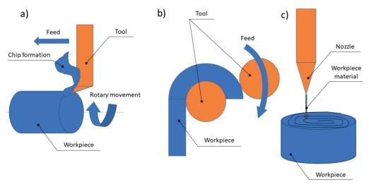
Fig. 1.18. Exemplery manufacturing processes: a) subtractive b) forming, c) additive
