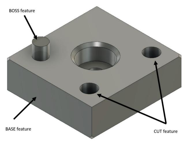
Fig. 1.8. An example of a solid model
