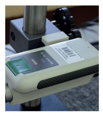
Fig. 1.46. Measuring system dedicated to measurements of roughness mainly under industrial conditions
