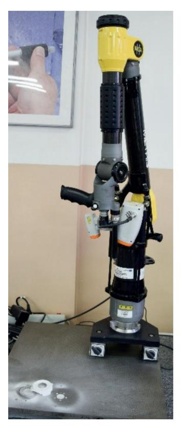
Fig. 1.48. Articulated measuring arm enabling contact and non-contact coordinate measurements and the reverse engineering process
