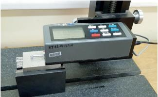
Fig. 1.27. INNOVATEST Surface roughness tester TR-220
