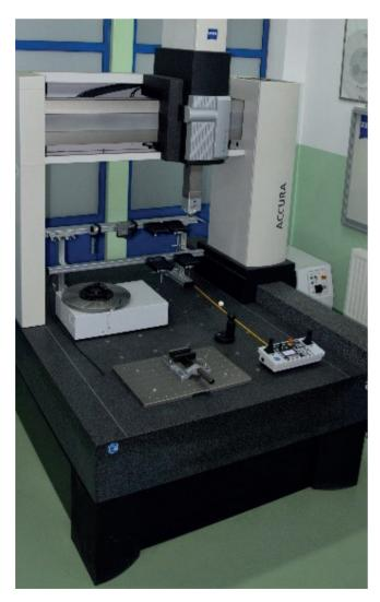
Fig. 1.51. Coordinate measuring machine ACCURA II
