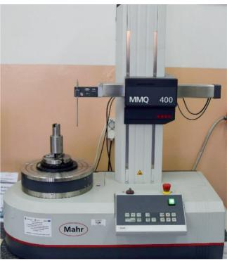
Fig. 1.49. Form measuring system MMQ 400 of the Mahr company applied for measurements of geometrical deviations of products
