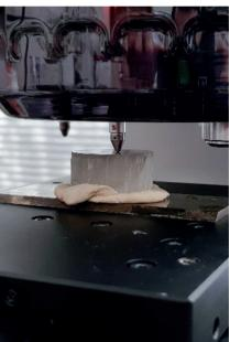
Fig. 1.30. Mitutoyo HM-200 Micro hardness testing machine
