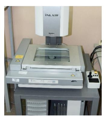
Fig. 1.44. iNEXIV measuring system mainly dedicated to 2D non-contact measurements
