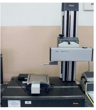
Fig. 1.45. MarSurf GD 120 dedicated to measurements of roughness of an object
