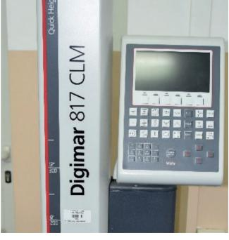
Fig. 1.43. Heigh measuring instrument produced by the Mahr company
