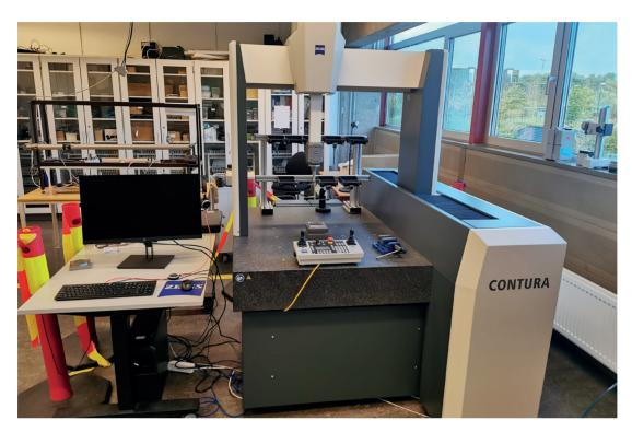
Fig. 1.57. Zeiss Contura Coordinate Measuring Machine
