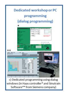
Fig. 1.16. Methods of CNC programming (based on figures from R. Wdowik's master thesis, Rzeszów University of Technology, 2009, and general division of programming methods)
