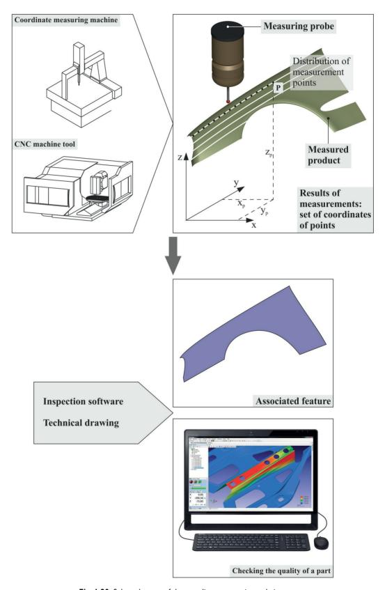
Fig. 1.20. Selected stages of the coordinate measuring technique
