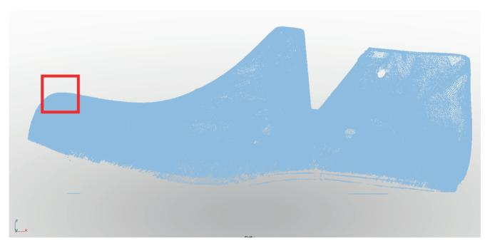
Fig. 1.9. Point cloud represantation of a physical object. Here there are close to I million points in the model
