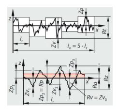
Fig. 1.29. Surface roughness profile measurements
