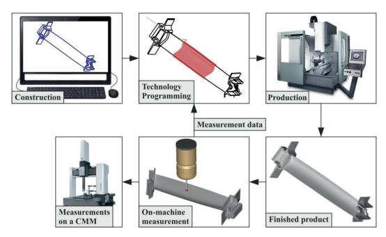
Fig. 1.22. On-machine measurements in a production process
