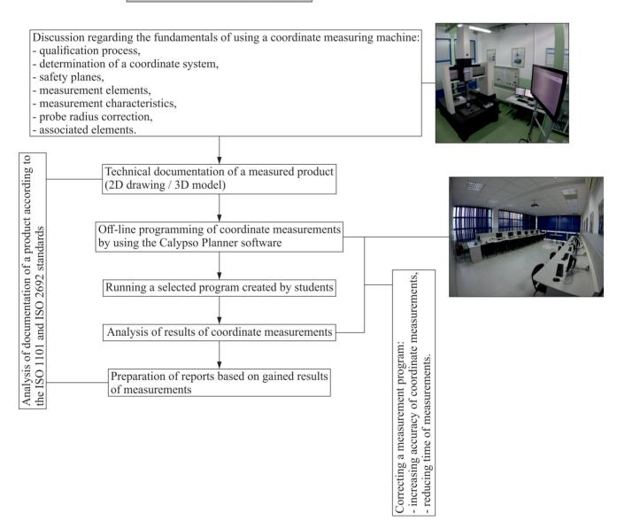
Fig. 2.15. Model of laboratory classes regarding the coordinate measuring technique
