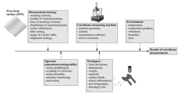
Fig. 1.23. Factors having the influence on the accuracy of coordinate measurements of, e.g. curvilinear surfaces of products [4]
