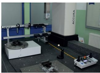
Fig. 1.52. Coordinate measuring machine ACCURA II equipped with three measuring probe and a rotary table
