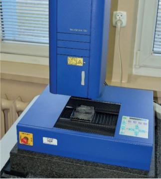
$\textbf{Fig. 1.50.} \ \, \textbf{TalyScan I50 dedicated to measurements of roughness}$
