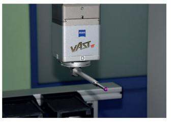
Fig. 1.53. VAST XT contact measuring probe
