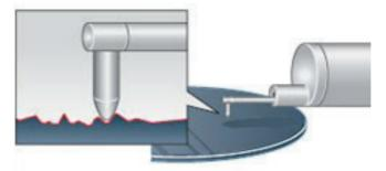
Fig. 1.28. Schematic illustration of surface roughness measurement
