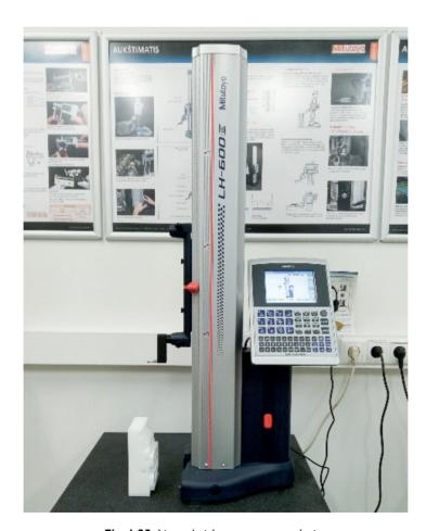
Fig. 1.25. Linear height measurement device
