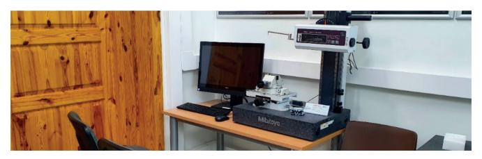
Fig. 1.40. Test-stand for surface quality analysis at Kaunas University of Technology
