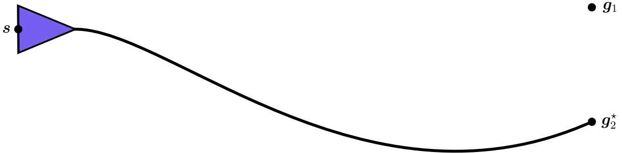
Figure 2.1: Example legible trajectory with respect to g_2^* , assuming g_1 and g_2^* are the robot's only goals in the workspace.
