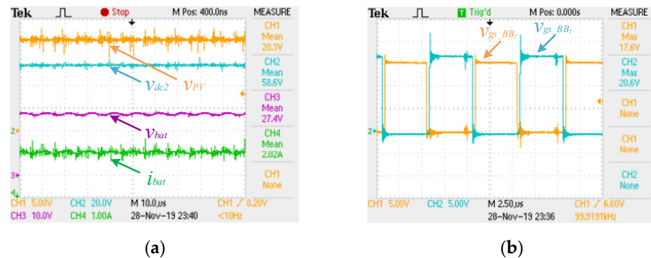
Figure 7. PV2B operation mode: (a) voltage on the solar PV panels (CH1: 5 V/div), secondary dc-link (CH2: 20 V/div) and BESS (CH3: 10 V/div) and current at the BESS (CH4: 1 A/div); (b) gate-source voltage in each of the semiconductors that make up the back-end bidirectional dc-dc buck-boost converter (CH1: 5 V/div), (CH2: 5 V/div).
