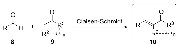
Scheme 1. Synthesis of chalcones with the Claisen Schmidt condensation.
