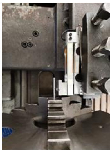
Figure 1. Top view of the contact between the Co28Cr6Mo and the WC cylinders.
