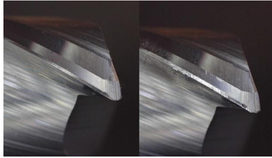
Figure 1. Cutting tool edge coated with TiSiN/TiSiVN during dry machining of CK45. Tool condition monitoring of the cutting edge to evaluate the performance of the tool.
