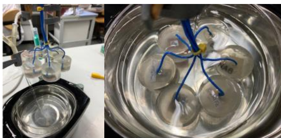
Figure 1. Setup of the corrosion cavitation test, before (left), and during the test (right)
