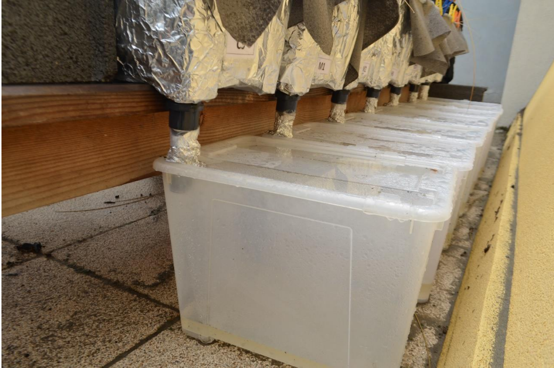
Figure 10. Free-draining systems isolated with aluminum sheets and connected through a pipe to individual containers that retain water runoff.
