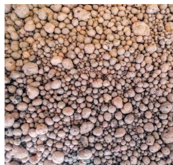
Figure 4. (a) Example of a drainage modular panel (source: Zinco, n.a.); (b) A granular material: light expanded clay aggregates (source: MIKE WYE, n.a )
