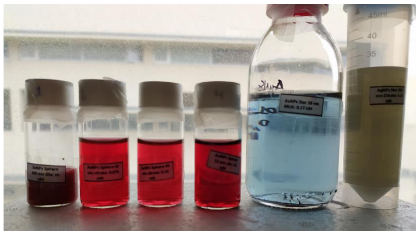
Figure 5 – Nanoparticles. From left to right: selenium nanoparticles, 60 nm gold nanoparticles, 40 nm gold nanoparticles, 12 nm gold nanoparticles, gold nanostars and silver nanostars.
