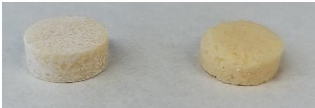
Figure 44. Tablets used in the dissolution test: on the left the tablet before the test and on the right after the test.
