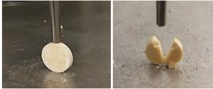
Figure 32. Hardness test using a Texture Analyzer.
