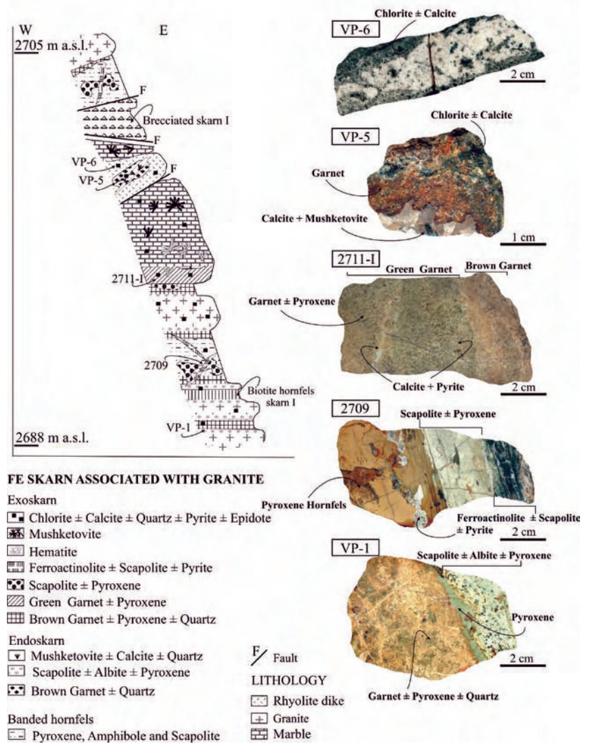
Fig. 15. Schematic E–W profile of the Fe skarn associated with granite and rhyolite, including photographs of the main alteration and mineralization styles in the profile. Sample VP6: chlorite ± calcite alteration of a rhyolite dike. Sample VP5: brown garnet ± quartz endoskarn partially altered to chlorite ± calcite with calcite ± mushketovite-rich pockets. Sample 2711-I: contact between proximal brown garnet ± pyroxene and distal green garnet ± pyroxene exoskarn zones cut by late calcite ± pyrite veinlets. Sample 2709: scapolite ± pyroxene exoskarn in pyroxene hornfels cut by late ferroactinolite ± scapolite ± pyrite vein. Sample VP1: contact between the scapolite ± albite ± pyroxene endoskarn in rhyolite and the brown garnet ± pyroxene ± quartz exoskarn with late calcite ± pyrite. A thin pyroxene envelope separates both zones.
