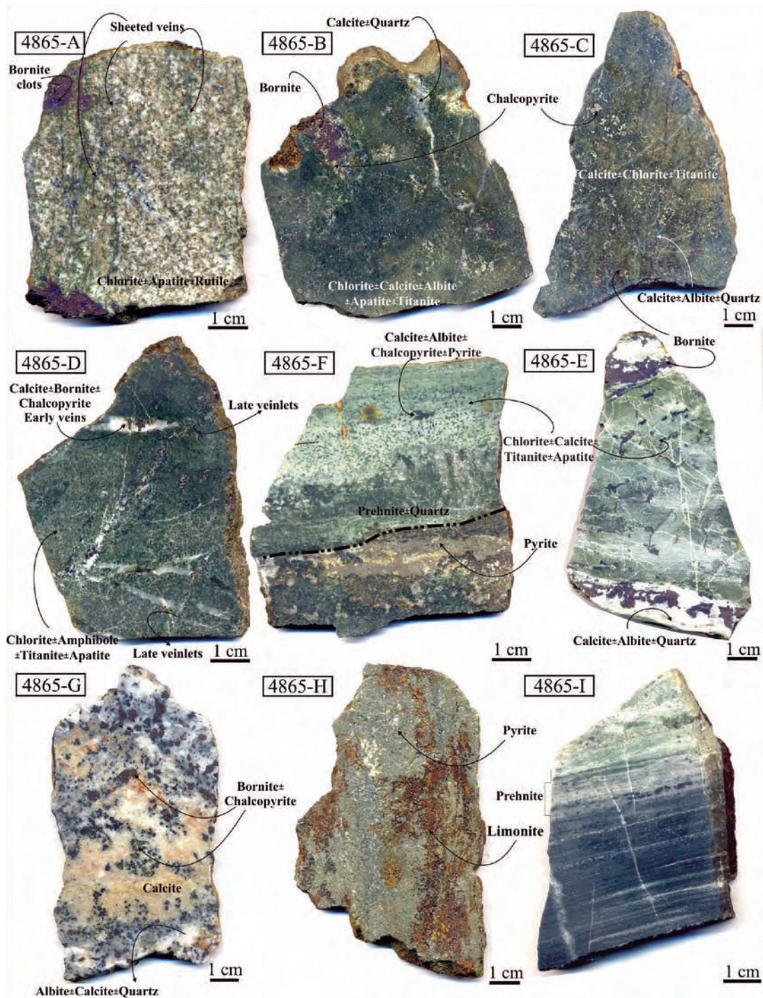
Fig. 19. Photographs of different alteration styles in diorite, siltstone, and limestone in the 3170 m elevation adit. Sample 4865-A: Altered diorite with a swarm of parallel fractures resembling sheeted veins, filled with calcite ± quartz ± bornite ± chalcopyrite and a green chlorite alteration envelope; these veinlets connect bornite clots. Samples 4865-B and -C: Intensely altered diorite with more than one generation of very thin sinuous calcite veinlets that connect disseminated bornite ± chalcopyrite grains, and thin bornite ± chalcopyrite veinlets with calcite ± albite ± quartz envelopes. Sample 4865-D: Early thicker veins with parallel walls, lenticular veins with calcite ± bornite ± chalcopyrite infill, and a colorless albite alteration envelope are cut and offset by bornite ± chalcopyrite, albite, and calcite veinlets. Sample 4865-E: Calcite ± bornite ± chalcopyrite ± albite ± quartz alteration has invaded early calcite ± chlorite ± titanite ± apatite alteration of siltstone along laminations (thick veins) and fractures (thin veinlets). Sample 4865-F: Late stage of calcite ± bornite ± chalcopyrite ± albite ± quartz veins. Sample 4865-G: Outer pyrite-rich zone with Co anomalies. Sample 4865-I: Alteration zone with prehnite and calcite ± chlorite ± rutile ± apatite and bornite ± chalcopyrite passes gradually to a fresh laminated limestone with clastic intercalations cut by late calcite veins.
