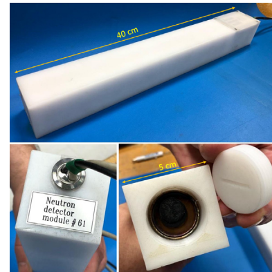
Fig. 5. Photos of a UNLV He-3 neutron detection module. We have secured 64 such modules for the NEMESIS upgrade.
