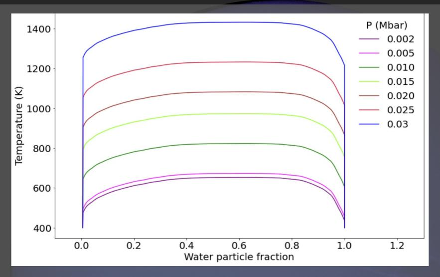
Provide demixing curves  $T_{dmx}(P, x_{H20})$
