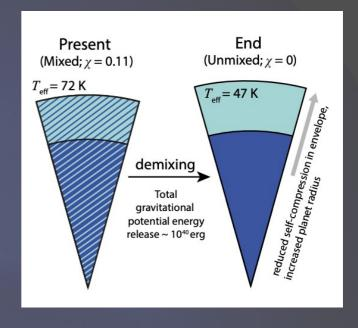
Find: H<sub>2</sub>-H<sub>2</sub>O demixing explains layered structure and could slow down Neptune's cooling rate. Different states of H<sub>2</sub>-H<sub>2</sub>O demixing can account for difference in heat fluxes between U. and N.
