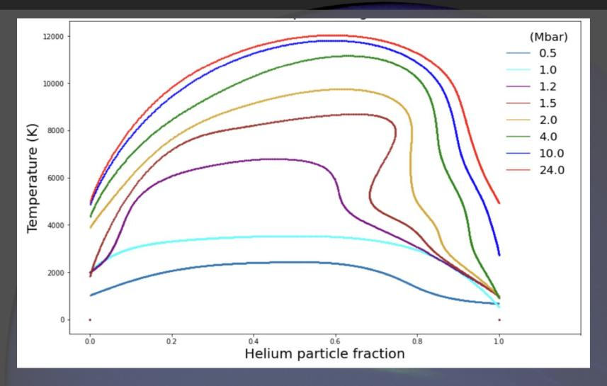
Demixing curves  $T_{dmx}(P, x_{He})$  provide the maximum temperature below which phase separation occurs
