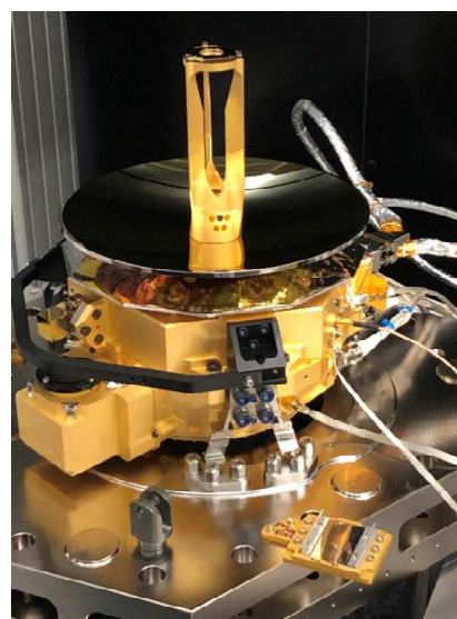
Figure 1. Top: The compact design of the GALA Transceiver Unit (TRU) [1] has been optimized for energetic-particle shielding of radiation-sensitive components such as the APD placed onto the focal plane in the centre of the instrument. The analogue active Q-switch electronics are located very close to the APD although their 10 ns switching spikes with amplitude 3 kV are electrically well shielded. The pump diode lasers are driven by current pulses with amplitude of 200 A that last about 70 \mu\text{s} . Bottom: Flight model of the GALA TRU on the test bench at Hensoldt Optronics in Oberkochen, Germany. Credit: DLR / Hensoldt Optronics / JAXA
