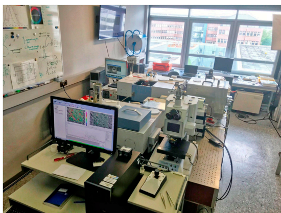
FIGURE 1 PSL configuration - Bruker Hyperion 2000 in the front right with a meteorite sample, on the left three Bruker Vertex 80V spectrometers with internal vacuum sample chambers, UV to FIR detectors, beamsplitter and sources and in the back a portable XRD system (orange box).
