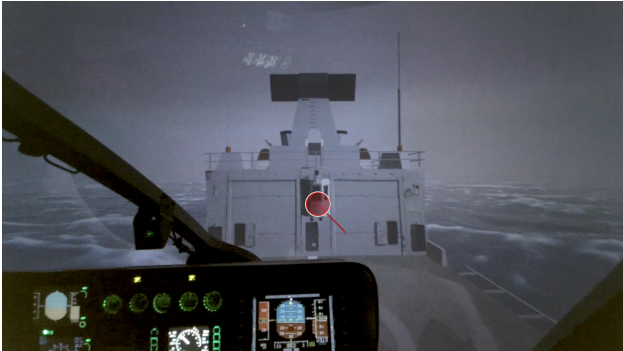
Figure 1 Final approach during a ship deck landing on the F-124 frigate in the AVES simulator with eye gaze (red circle)
