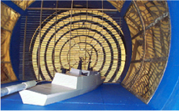
Figure 5 Ship air-wake measurements at IMFL wind tunnel facilities
