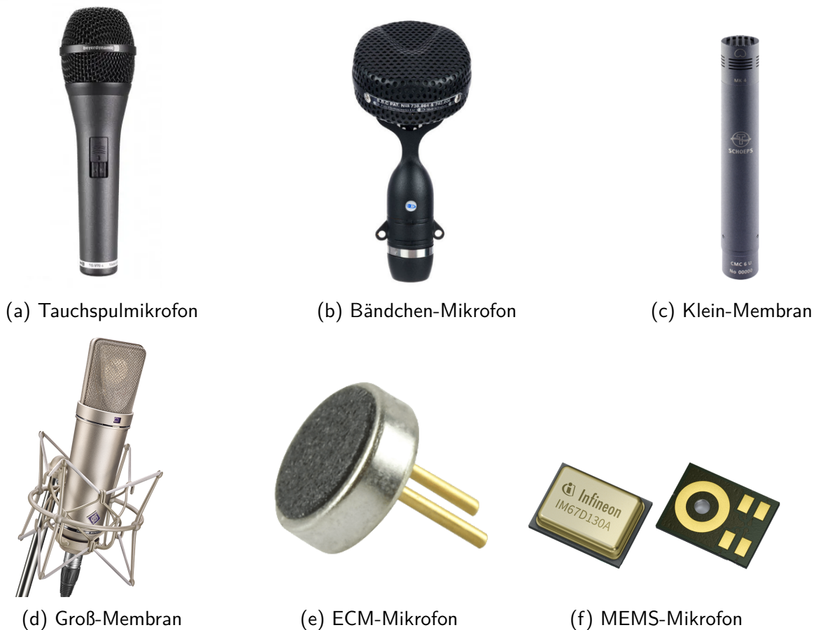
Abbildung 2.3: Unterschiedliche Mikrofonarten. a) Beyerdynamic TG V70 [Bey21] b) Coles 4038 Studio Ribbon [Tho21] c) Schoeps Colette CMC-64 [Sch21] d) Neumann U 87 Ai Studio Set [Neu21] e) CUI Devices CMC-4012-40P [CUI21] f) Infineon IM67D130A [Inf21]
