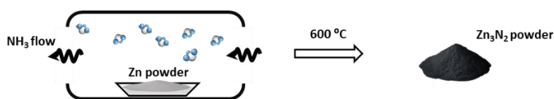
Figure 41 Schematic illustration of the synthesis of Zn 3 N 2 powder.
