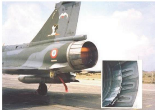
Figure 3 – Ceramic matrix composite of C/SiC components on the Snecma M53-2 aircrafts' engine (Bansal & Lamon, 2014).
