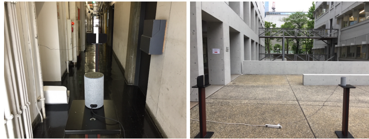
Fig. 2.18 Experiments in a hallway (left) and outside (right). We install the parametric loudspeaker and smart speaker at the same height. The detail result was presented in Sec 5.1.2, Table 2.
