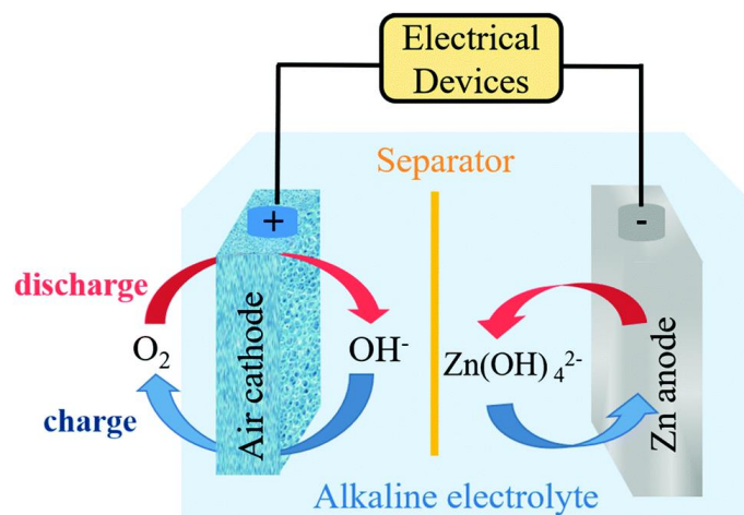
Figure 1.4. Schematic of a typical rechargeable Zn negative electrode (anode) battery [50]. Republished with permission of Royal Society of Chemistry, from Challenges, Mitigation Strategies and Perspectives in Development of Zinc-electrode Materials/Fabrications for Rechargeable Zinc-air Batteries, J. Yi, 11, 2018; permission conveyed through Copyright Clearance Center, Inc.
