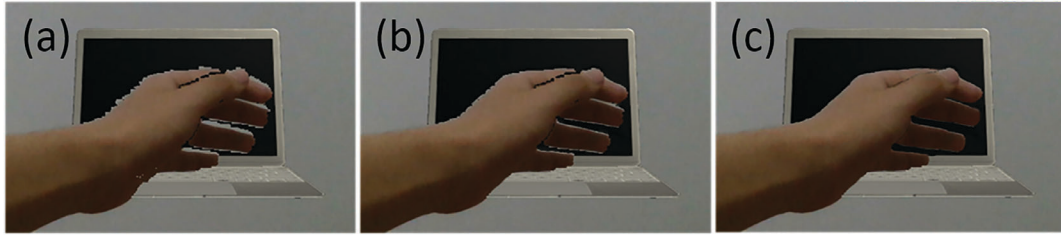
FIGURE 3.9: A mixed reality scene rendered with occlusions based on (a) naive approach that uses raw depth, (b) CVF occlusion [102] and (c) our approach.
