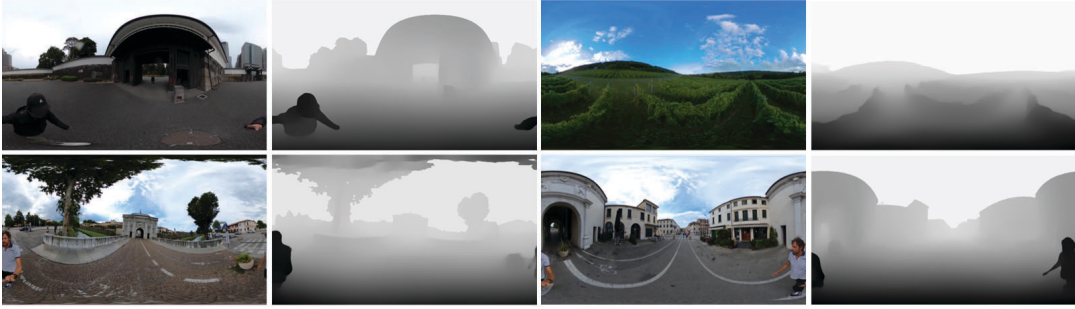
FIGURE 5.3: Examples of generated RGB/depth pairs. The color images are video frames acquired from the internet, and the corresponding depth maps is generated through our test-time training method.
