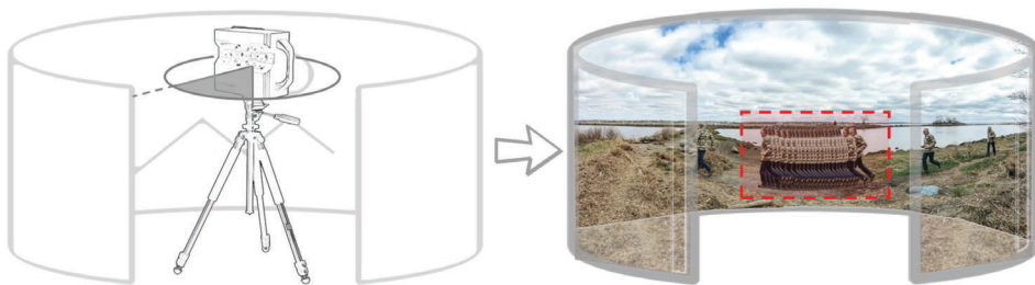
FIGURE 4.1: A demonstration of incorrect representations of dynamic objects (e.g. a running person) captured with an omnidirectional RGBD scanning device.
