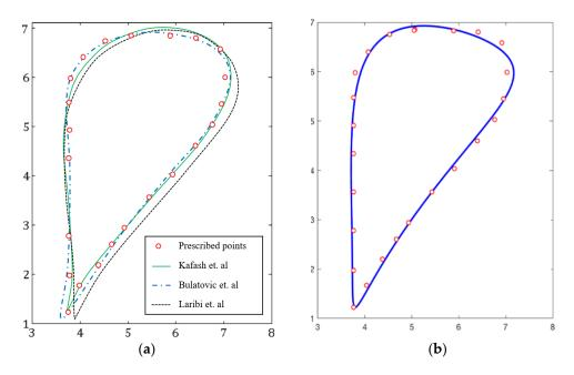
Figure 10. Example 2: optimal solution for: (a) four-bar and (b) slider-crank mechanism.
