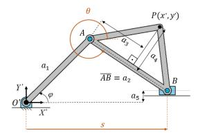
Figure 1. Slider-crank mechanism with 5 dimensional parameters.
