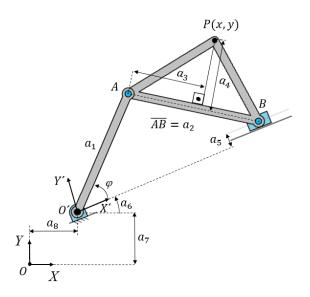
Figure 3. Slider-crank mechanism with 8 dimensional parameters.
