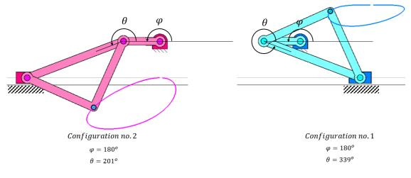
Figure 2. Two possible configurations for the same input.
