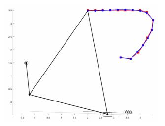
**Figure 8.** Example 1: best multi-start solution for slider-crank, E = 0.0073.
