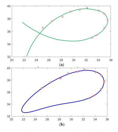
**Figure 11.** (**a**) Watt's mechanism optimal solution from [41]; (**b**) optimal solution for slider-crank mechanism.
