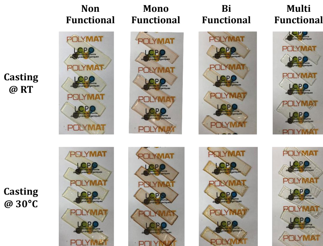
Figure 8: Pictures of the cast films at RT and 30°C of hybrid-PHUs of different architectures (20wt% PHU in all the cases)
