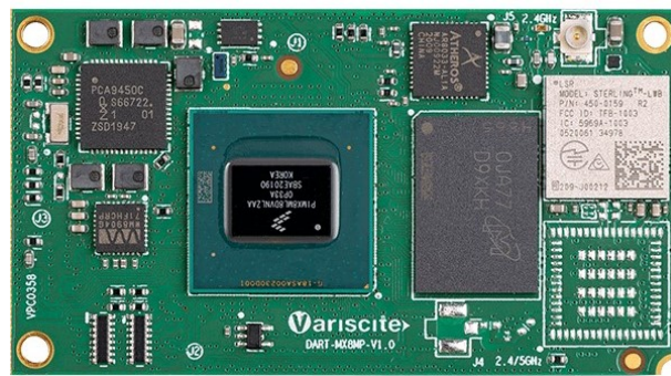
Figure 1. iMX 8M Plus System on Module. Image from https://www.variscite.com/ (accessed on 2 September 2021).
