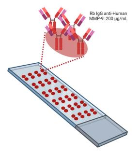
**Figure 7.** Schematic representation of a microscope glass slide with AbMAs printed. Twenty-four AbMAs with two spots of rabbit IgG anti-human MMP-9 at 200  $\mu$ g/mL in SIVG 0.05% were immobilized onto treated slides. Image created with BioRender.com.
