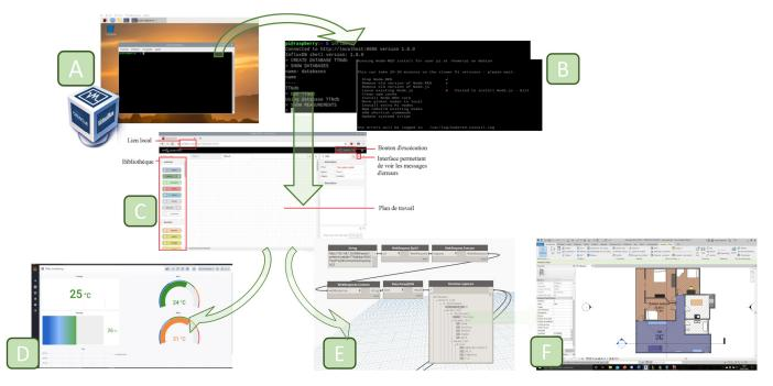
**Figure 7.** Workflow followed by the students under the RVL methodology during the project development. (**A**): Raspberry Pi OS simulated under VirtualBox, (**B**): Command-line interface of Raspberry Pi OS, (**C**): Node-RED environment, (**D**): designed dashboard in Grafana, (**E**): developed script in Dynamo, (**F**): Revit model.
