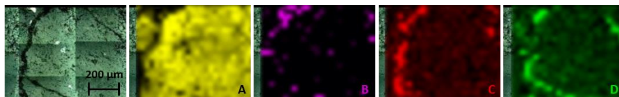
Figure 1 : High Resolution Raman images of (A) Olivine, (B) Pyroxene, (C) Epsomite and (D) Gypsum along the RBT 04262 Mars meteorite.
