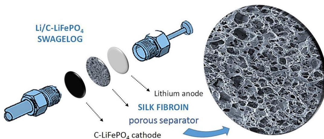
Figure 5.2. 3. Schematic representation of the Swagelok cell type and its components.
