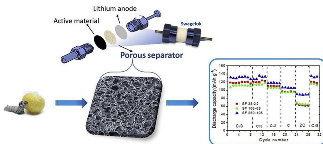
Figure 5.2. 1. Graphical abstract of porous SF membranes for Li-ion batteries separator.
