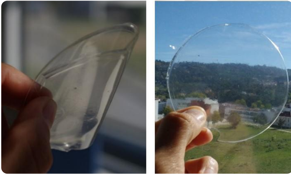
Figure 2. 10. SF films with mechanical flexibility and optical transparency.
