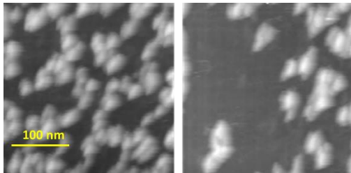
Figure S3.2. Tetramers directly attached to Mica surface visualized by HS-AFM, before (left) and after \text{Ca}^{2+} addition (right).
