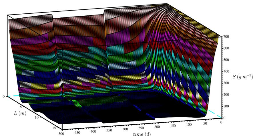
Fig. 12. Evolution over time and longitudinal position of the substrate concentration during the rainy season.
