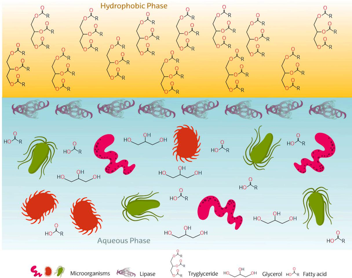
Fig. 2. Schematic representation of the grease trap interface.
