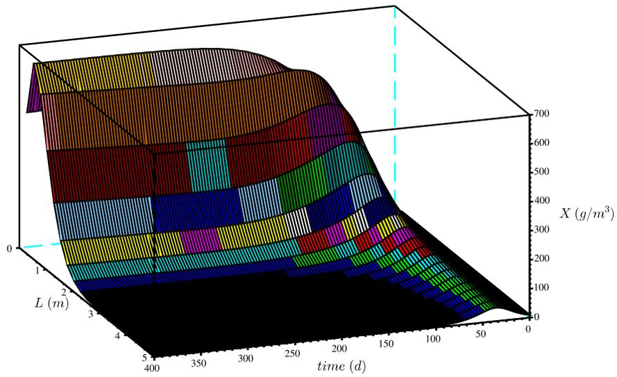
Fig. 7. Evolution over time and longitudinal position of the microorganism concentration.
