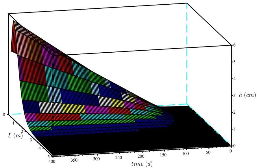
Fig. 8. Evolution over time and longitudinal position of the height of the sludge layer in the gravel bed.
