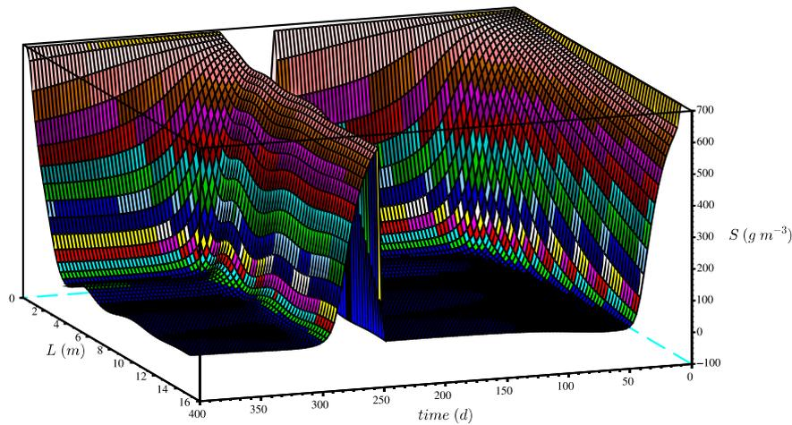
Fig. 10. Evolution over time and longitudinal position of the substrate concentration during the holiday shutdown.
