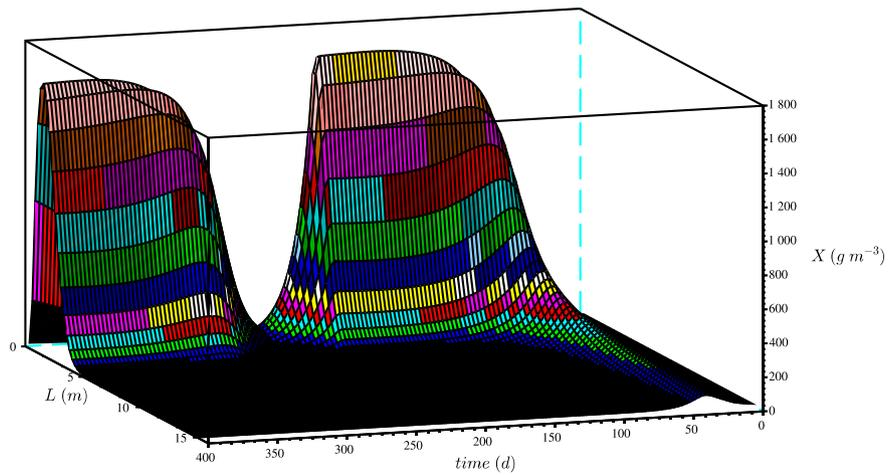
Fig. 9. Evolution over time and longitudinal position of the microorganism concentration during the holiday shutdown.
