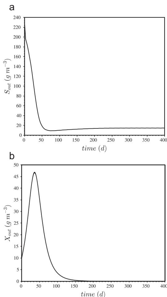
**Fig. 5.** Evolution of the a) substrate and b) microorganism concentrations at the end of the gravel bed over time.
