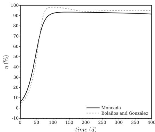
**Fig. 4.** Evolution over time of the removal efficiency in the simulations of constructed wetlands, as studied by Moncada [56] and Bolaños and González [57].
