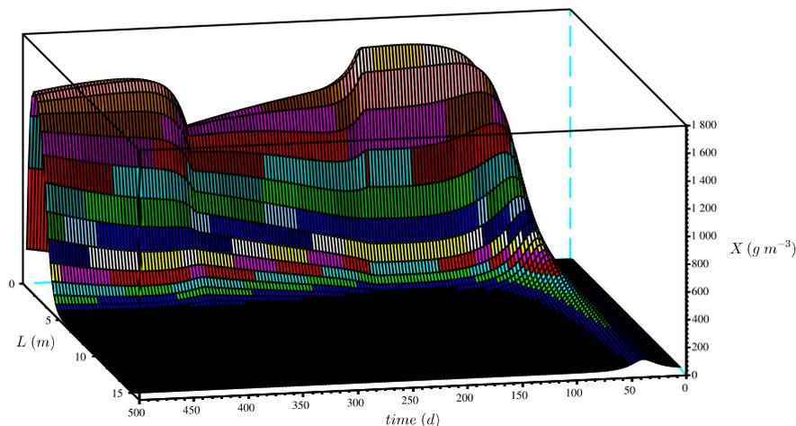
Fig. 11. Evolution over time and longitudinal position of the microorganism concentration during the rainy season.
