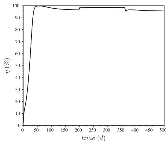
Fig. 13. Evolution over time of the substrate removal efficiency during the rainy season.
