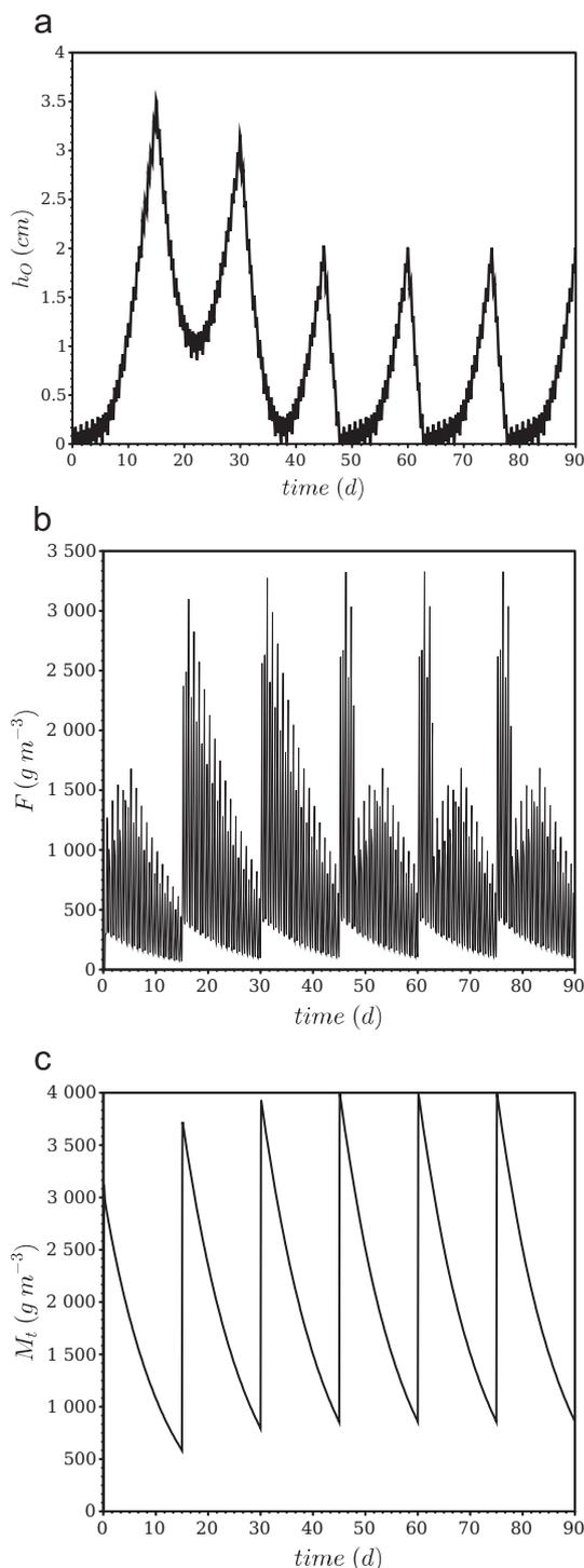
**Fig. 3.** Evolution over time of a) the height of the fat and oil layer, b) the concentration of fatty acids and glycerol in the aqueous phase, and c) the microorganism concentration.
