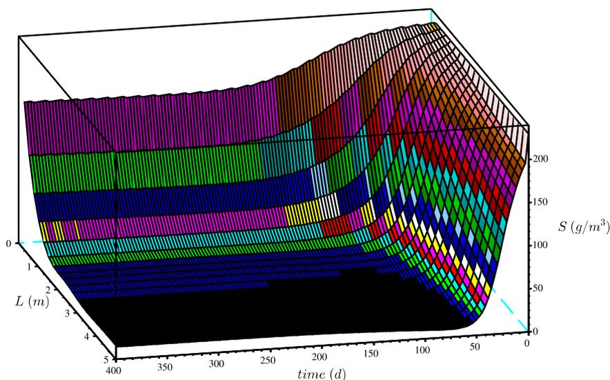
Fig. 6. Evolution over time and longitudinal position of the substrate concentration.
