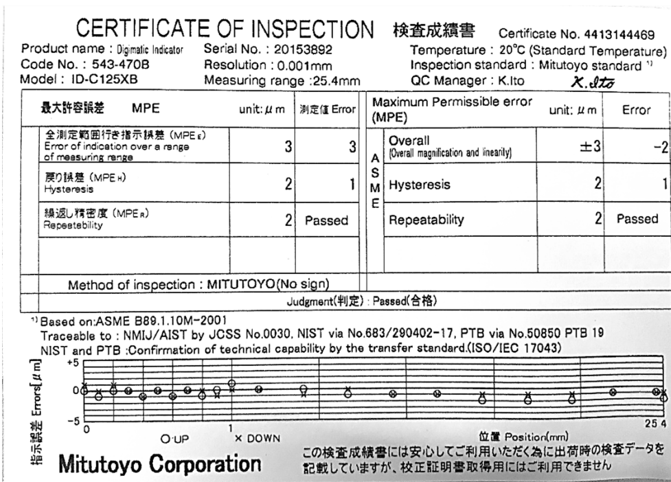
Figure D.2 Certificate of inspection of the dial indicator serial number 20153892.
