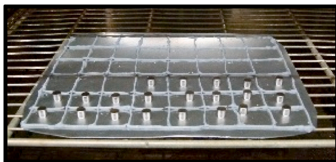
Fig. 2. Sample rack with some of the samples inside the heating cabinet.
