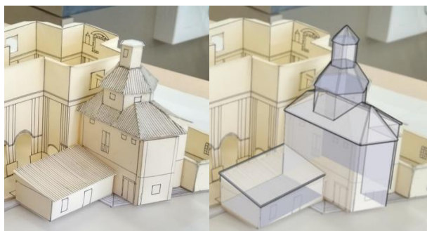
Figure 5: During the modelling, some of the solutions for the roofs of the mock-up were considered unrealistic and, hence, it was decided to modify them.
