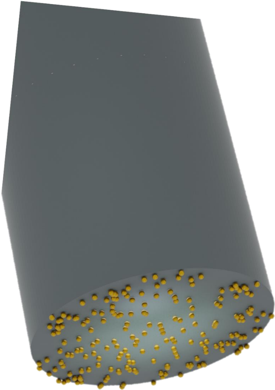
Figure 20. Sketch of typical lab-on-tip-based sensor based on a chemical immobilization of AuNPs.
