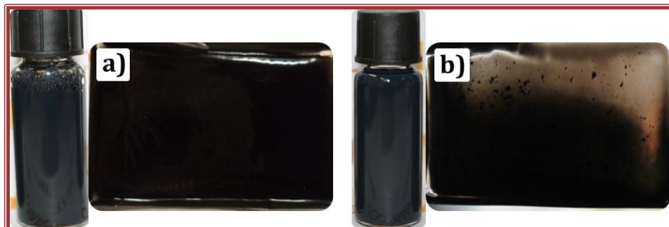
Figure III.7. Images of polymer films cast from a) hybrid dispersion containing 0.5 wt% air sonicated MWCNTs; b) hybrid dispersion containing 0.5% water sonicated MWCNTs.
