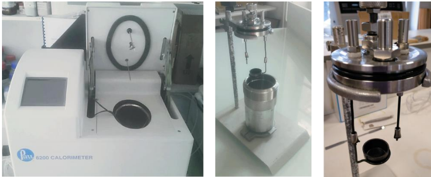
Figure 51. Calorimeter employed for the determination of the combustibility of the samples: a) Whole machine with the screen for the results and oval vessel with water in which the calorimetry pump is introduced, b) Calorimetry pump with pressurized sealing and releasing valves, c) Pan for the sample in contact with the wire, which created the spark for the combustion.
